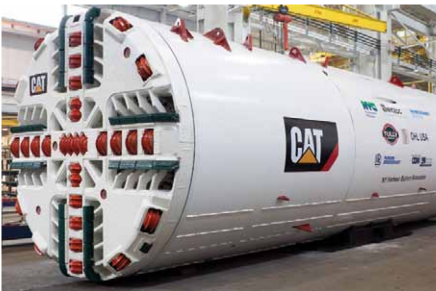
TBM (EPB - mix face)
